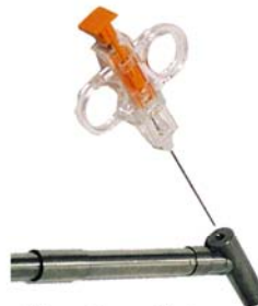
• Biopsy Gamma Probe Probe with a central opening for insertion of biopsy needle. Diameter = 14 mm.
